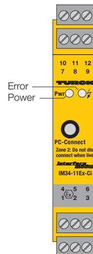
The 1-channel temperature measuring amplifier IM34-11EX-CI is designed to evaluate the temperature-dependent variations of resistance thermo detectors (RTD) Ni100/ Pt100, thermoelement types B, E, J, K, L, N, R, S and T or low voltages in a range of -160...+160 mV and to output them as linear temperature current signals.
